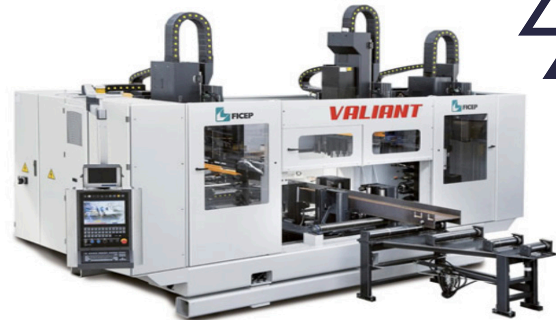
High-performance CNC machine for automated steel processing with dual drilling head
